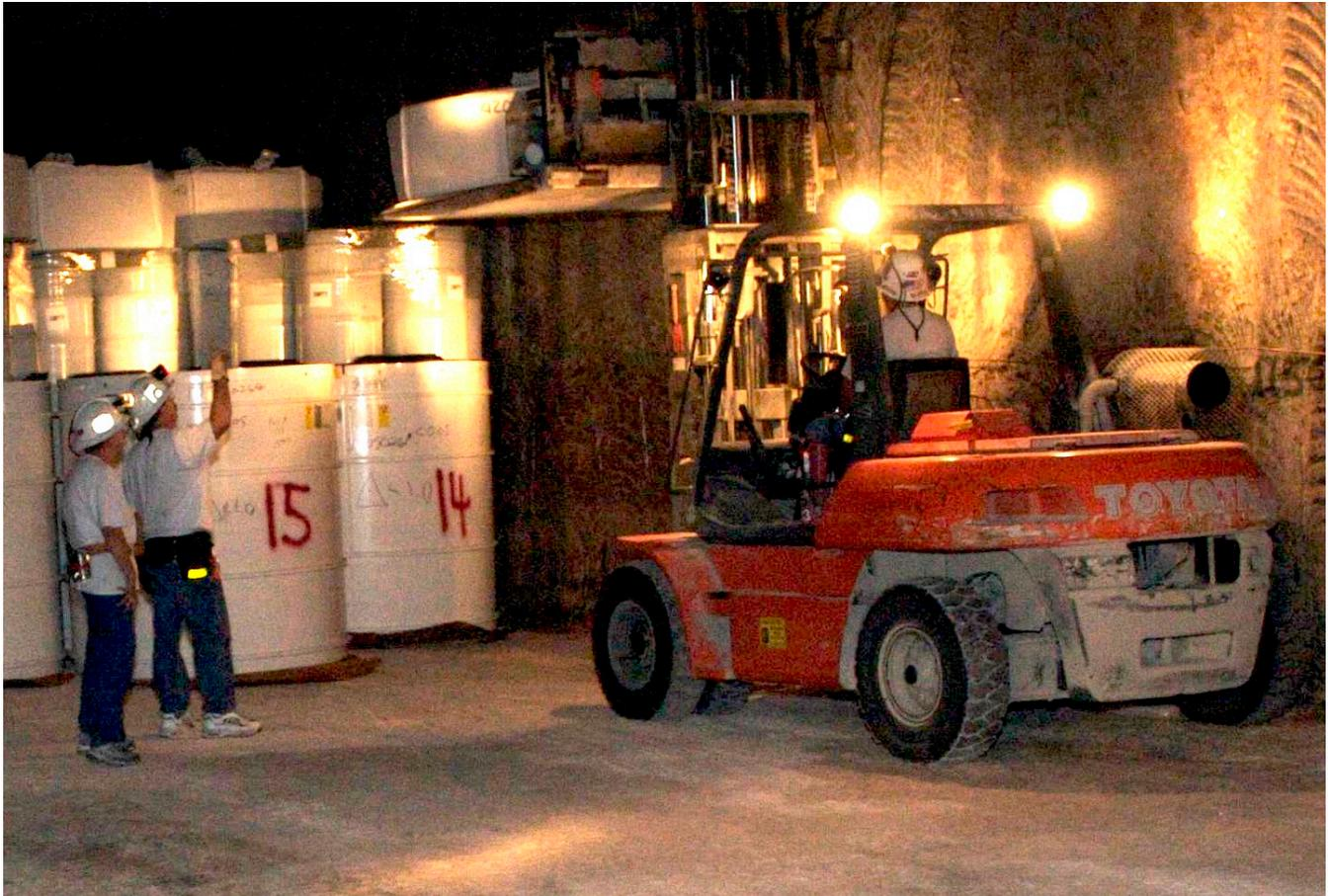
WIPP personnel place “super sacks” of magnesium oxide on the top of waste columns during underground waste disposal operations.
